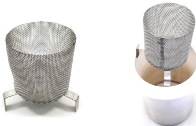
Figure 28. Metal container used to protect the molecular sieves from the magnetic stir bar.
