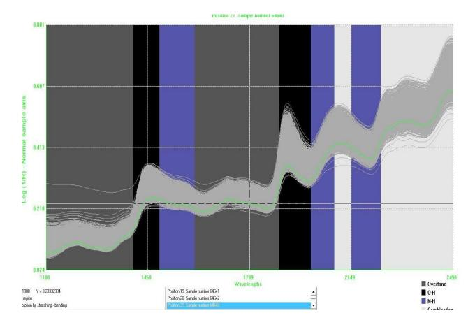
NIR spectra are plots of reciprocal  $log_{10}$  reflectance (log 1/R) versus the wavelength Figure 1. NIRS spectra data for chickpea haulms.
