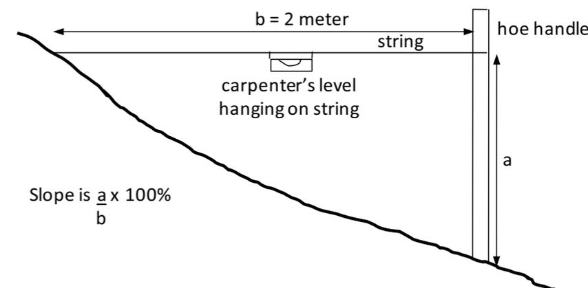
Figure 9. Simple method to determine slope using a line level.
