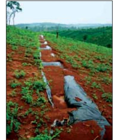
Photo 4. FPR erosion control trial
