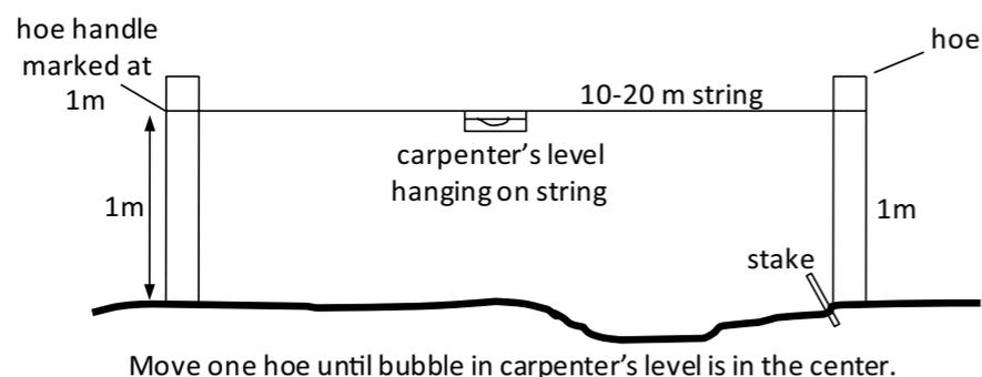
Figure 11. Simple method to set out contour lines using a line level.
