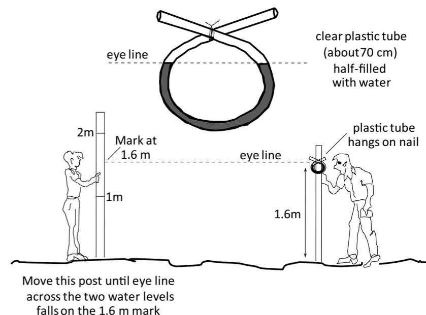
Figure 12. Simple method to set out contour lines using a plastic tube with water: the “buffalo horn”.
