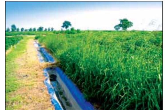
Photo 2. Soil erosion control experiment using plastic covered channels to collect eroded sediments
