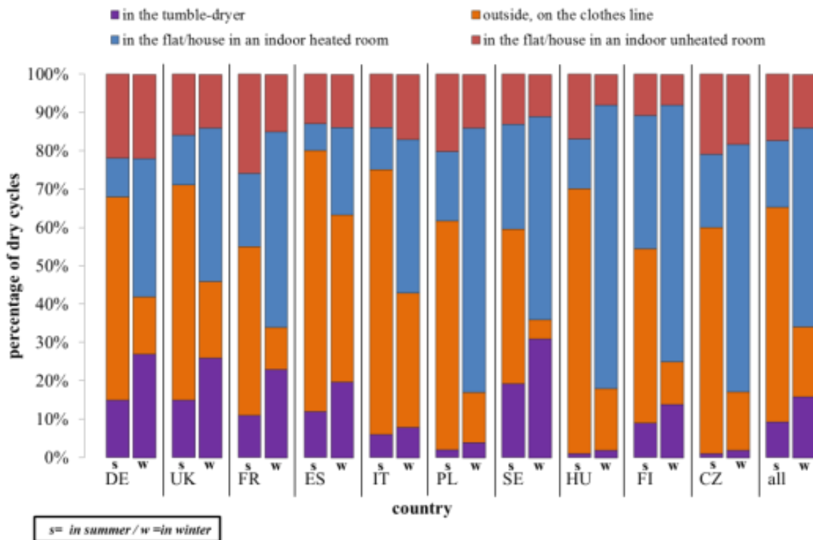
Figure 3.46: Method of drying the clothes in summer (S) and in winter (W) for different European countries in 2011 (according to (Schmitz & Stamminger 2014))
