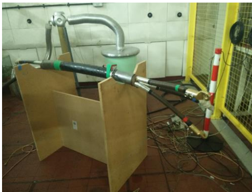
Figure 18. PD testing of 3core PILC cable
