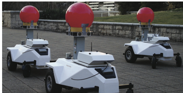
Figure 26: Three robots used for experimental evaluation of the leap-frog localization and coverage strategy.
