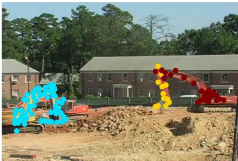
Figure 2.3: On the left an example of a rigid motion: an excavator is moving forward without moving its arm, hence, its motion is correctly classified as one motion (blue dots). On the right another excavator is rotating and at the same time is moving its arm, hence, this is an articulated motion correctly segmented in its two motion components (yellow and red dots). Image adapted from [31].
