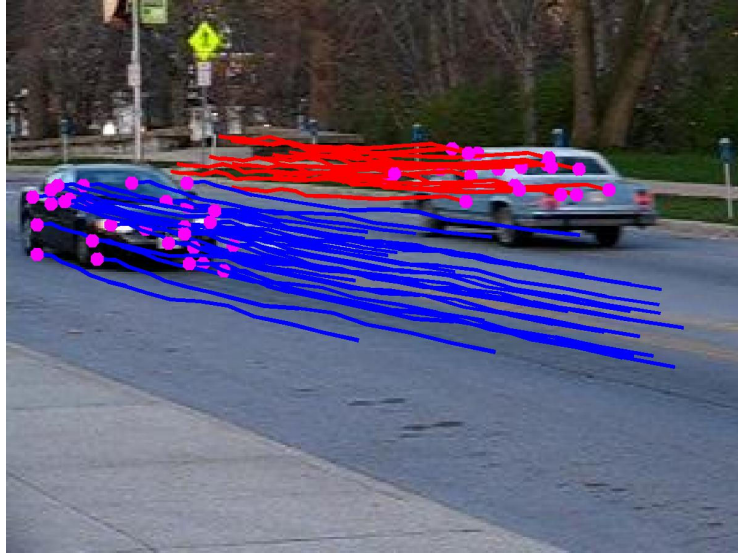
Figure 3.1: Example of an LSA result applied to a video sequence. Blue and red represent different labels, and therefore, different motions. The pink dots are the tracked features extracted from the first video frame. Sequence cars2_06_g12 of the Hopkins155 database.
