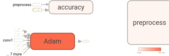
Figure 5-1: Part of the graph of the fully convolutional network. More demanding nodes, in terms of computation time, appears more reddish
