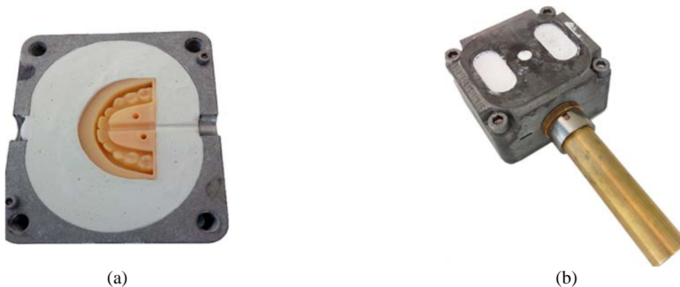
Fig. 14: (a) Mould enclosed in a plaster block before the silicone injection, (b) system ready for the injection process.
