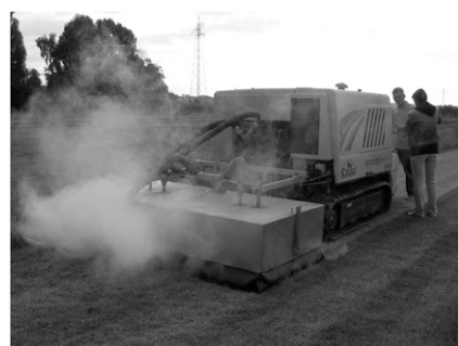
Fig. 1. Steaming machine during a treatment for cool-season turf control.
