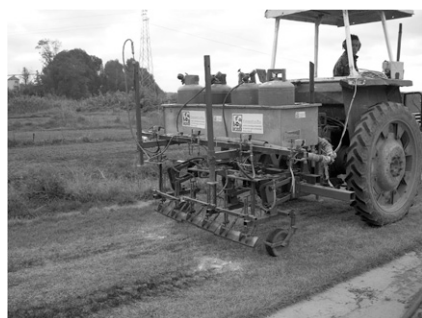
Fig. 2. Flaming machine during a treatment for cool-season turf control.
