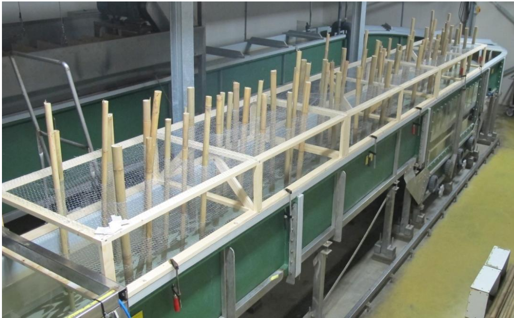
Figure 3.1: Mimicked mangrove roots used in our flume experiments. Bamboo sticks (0.04 and 0.06 m diameter) were more or less regularly interspersed over the whole length of the construction, mimicking 3 different root densities (10, 20 and 30 roots m -2 ). For technical details on the flume, see Bouma et al. (2005).
