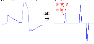
Figure 7. Single edge followed by a pulse having positive amplitude.
