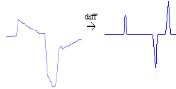
Figure 8. Single edge followed by a pulse having negative amplitude.
