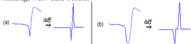
Figure 9. Abrupt fall before initial edge. (a) Pointed. (b) Round.
