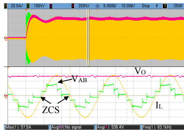
Figure 15. Evolution of voltage V_{AB} [100 V/div] output voltage V_O [200 V/div] and current I_L [20 A/div] in the multilevel LCC converter with a load R_O = 88.5 \Omega , P_O = 3.6 kW.
