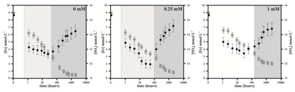
Figure 1: Evolution of (squares) Fe and (circles) SO<sub>4</sub> concentrations in a representative batch experiment, with As-free solution, 0.25 and 1 mM [As] initial. Graphics are divided into three stages; nucleation, cluster growth and equilibrium (from white to grey).
