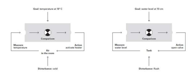
This diagram describes the general form of a negative feedback loop. It applies to toilets, thermostats, and other governors.
