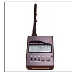
Figure 2 Frequency Detector [17]
