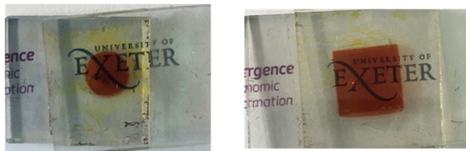
(a) Fabricated Bare DSSC (b) Scaled up DSSC
