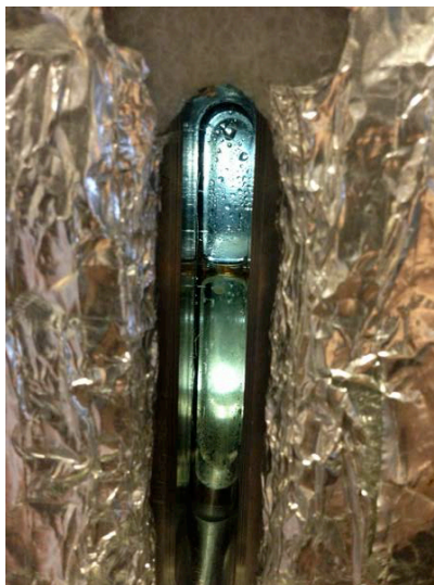
Figure 4.5 Image of 0.5 mass% PVCap with 2.0 mass% 1-octanol relative to water under 70 bar North Sea natural gas pressure at 20 °C in a visual autoclave cell (window is ~15 mm across). When mixing is stopped, the amber 1-octanol + PVCap phase gravity settles within a short timescale (almost fully clear in 10-20 minutes).
