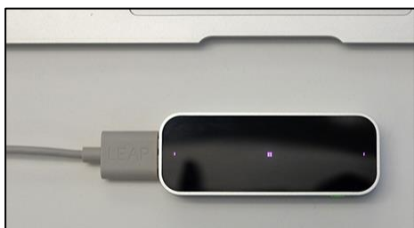
Fig 1. Leap Motion device connected to a laptop. The three IR LED's can be appreciated.
