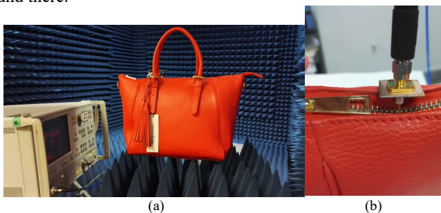
Fig. 19. Measurement of the reflection coefficients of the handbag zipper antenna with a vector network analyzer. (a) The scenario of the measurement. (b) The close-up of the feeding structure.
