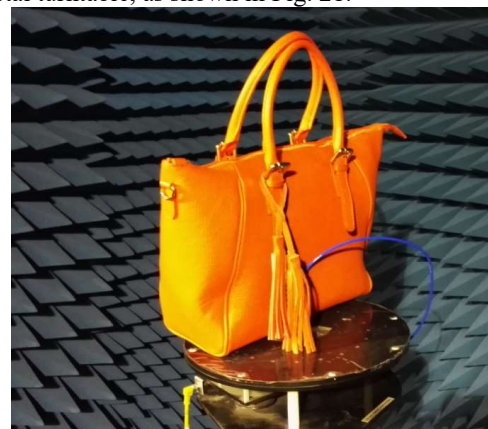
Fig. 21. Measurement of the radiation patterns of the bag zipper antenna in the anechoic chamber.
