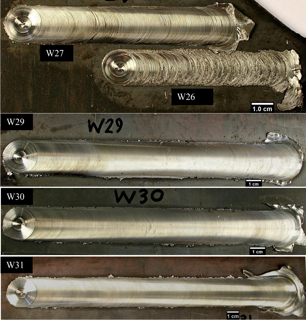
Figure 6.1 Optical macrograph of the BOP welds W26 and W27 and the butt FSW W29, W 30 and W 31.
