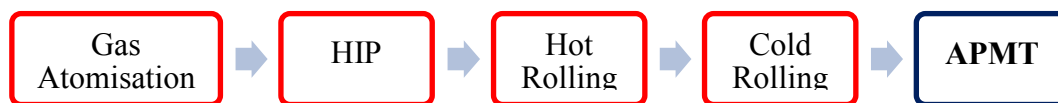
Figure 3.2 A schematic showing the different processing steps for the production of APMT alloy
