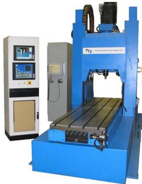
Figure 3.3 FSW machine model RM-2 used for all the welds at TWI Rotherham UK (Image TWI).
