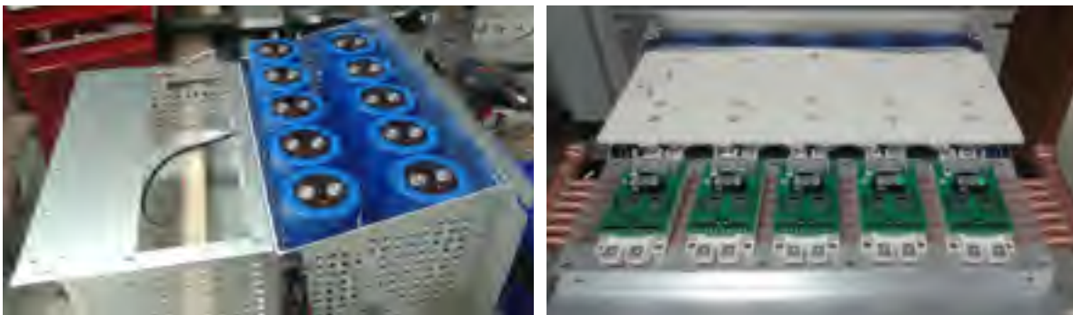
Figure 3.19 Capacitor bank, heatsink, and IGBT modules during assembly
