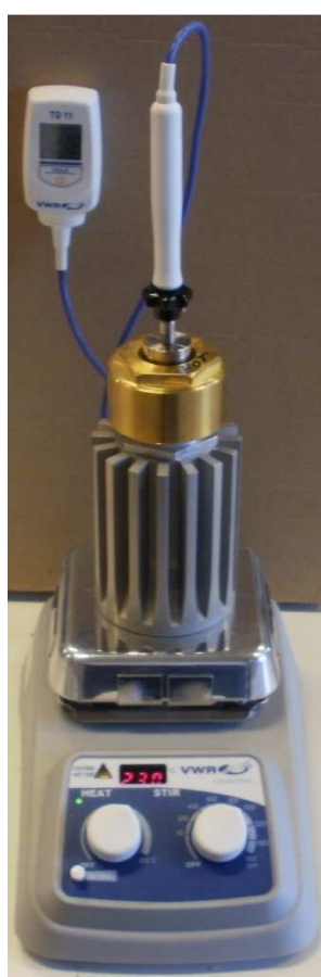
Figure S1. Pressure vessel for preparing amylose inclusion complexes.
