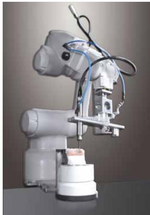
Figure 2. Device that drills hole in definitive cast and places implant analogue. Device is connected to computer, which has information from coded healing abutment.
