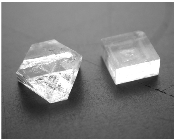
Figure 2.6 NaCl crystals grown from pure water (right) and water with some formamide. 24
