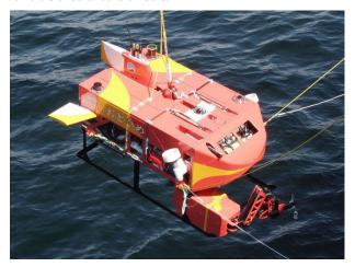
Figure 1. Autonomous Underwater Vehicle "Otohime".
