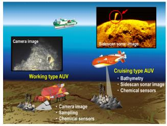
Figure 3. Oceanographic survey using AUVs.
