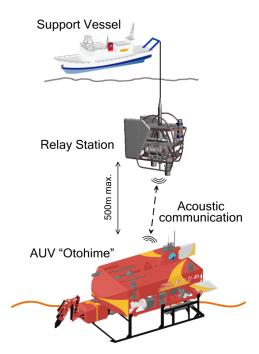
Figure 4. UROV operation based on acoustic communication using relay station.
