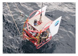
Figure 9. Deployment of the communication relay station for "Otohime".
