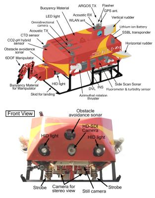
Figure 2. General arrangement of the "Otohime".
