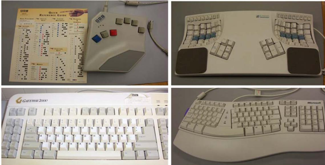
Figure 1: The four alternative keyboards used in this study: chord (top left), contoured split (top right), Dvorak (bottom left), split fixed-angle (bottom right).
