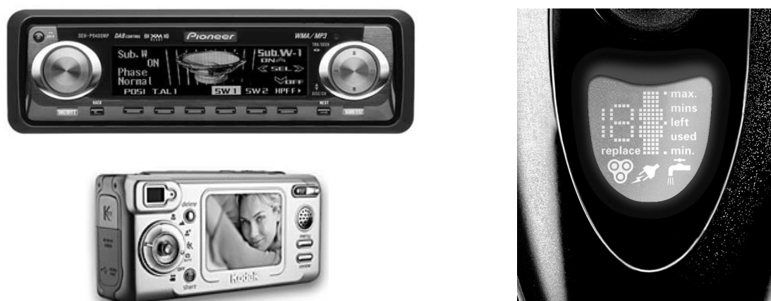
Figure 1.1 A selection of commercially available products, in which semiconducting organic moieties are employed. Top, left: Pioneer car radio with an oLED display. Right: Philips shaver with a pLED display. Bottom left: Kodak digital camera with an oLED display.
