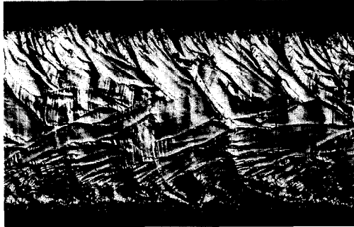
Figure 2. Optical micrograph of laser nitrided surface showing lamellae and ripples.
