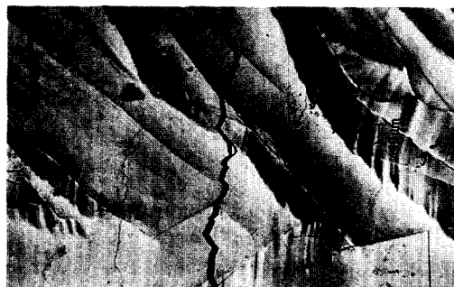
Figure 3. Optical micrograph showing microcracks with different orientations and one crack perpendicular to the scan direction.
