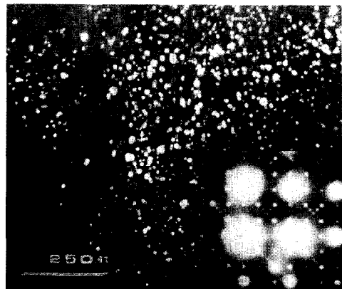
Figure 2. TEM micrograph of coherent precipitates in SQ-ASCM10 with its diffraction pattern.
