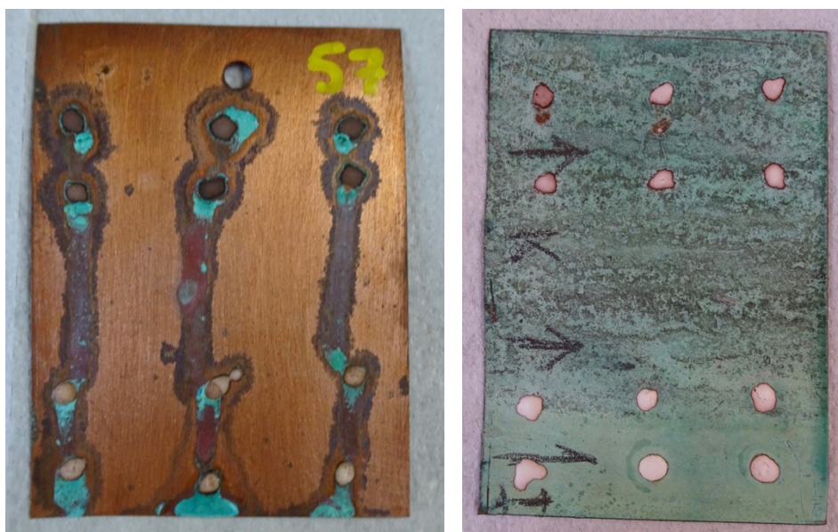
Figure 28: Example of samples removed from 2 weeks of exposure to RH + \text{SO}_2 . Uric acid + potassium chloride (C5) is dripping onto the uric acid + potassium sulphate (C6) on the copper sample, whereas no dripping can be seen on the roof sample
