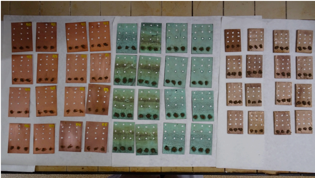
Figure 18: The copper, roof, and bronze samples with the first four contaminants applied
