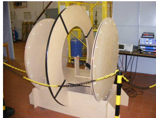
Fig. 7. Maxwell coils used to generate a uniform B -field in the laboratory.
