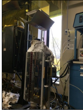
Figure 3.10: Thermogravimetric (TGA) analysis system for air/CO 2 reactivity of anode core samples at UQAC
