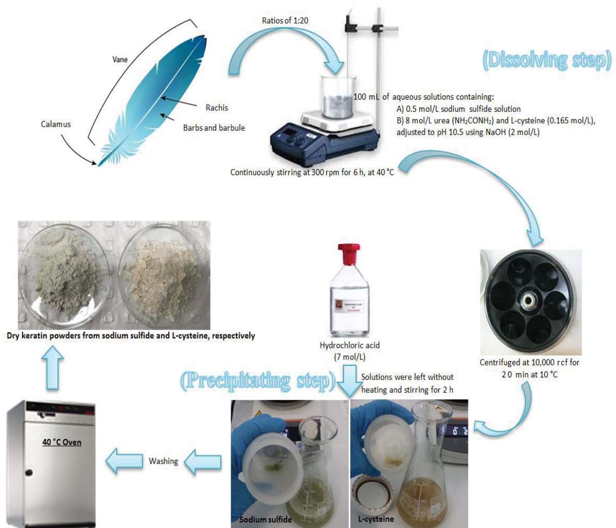
Figure 8.1: The extraction process of keratin from waste chicken feathers using sodium sulfide and L-cysteine
