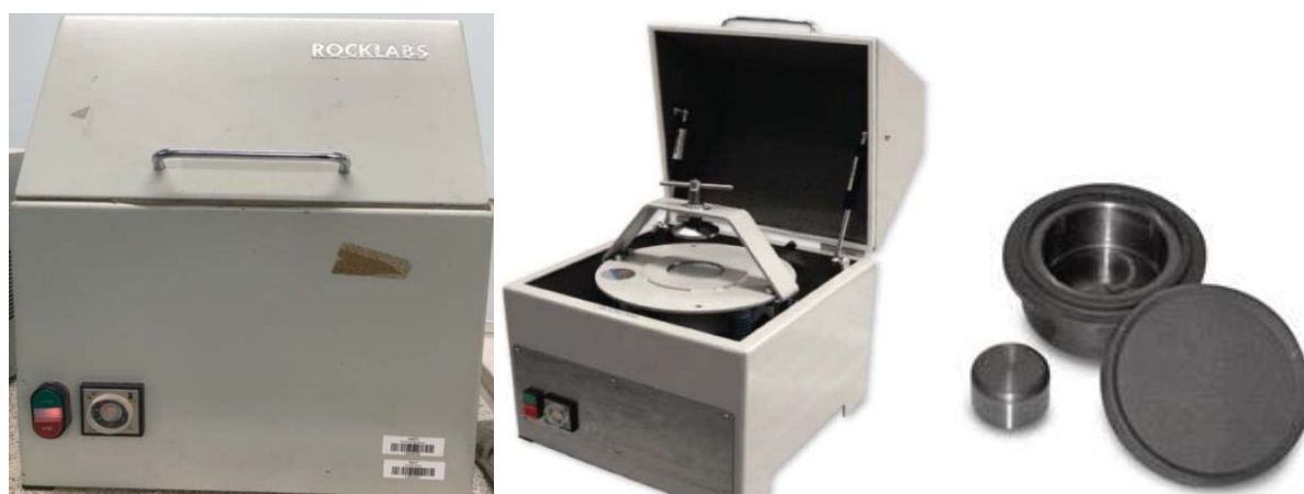
Figure 3.21: Rocklabs Ringmill Grinder, equipped with a zirconia mill head, grinding CFFs to powder form Rocklabs Ltd., Auckland, New Zealand
