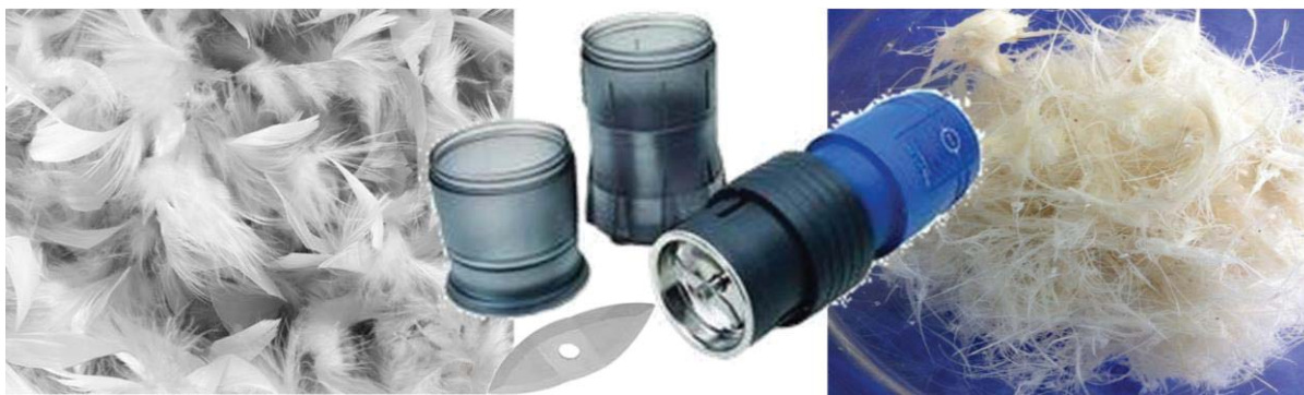
Figure 3.20: IKA ® A11 Crushing Analytical Mill, equipped with stainless steel cutting blades and inner tank, grinding CFFs to the size of 5 \mu\text{m} to 2 cm
