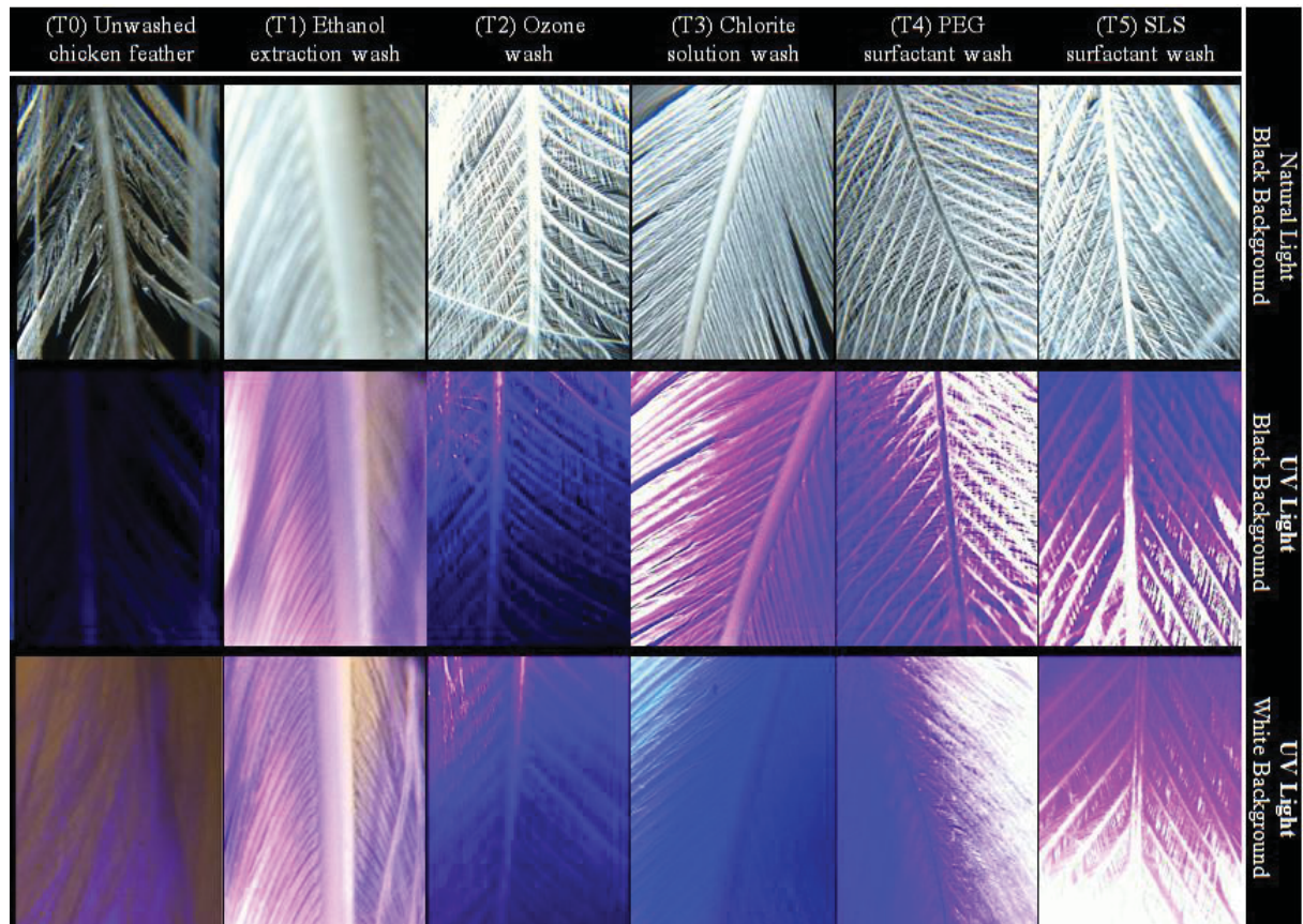
Figure 5.6: Chicken segments under natural and ultraviolet light at 80X magnification a) untreated chicken feathers upon receipt (T0), chicken feathers purified with b) SLS solution (T5), c) PEG solution (T4), d) SEEt treatment (T1), e) O 3 solution (T2) and f) ClO 2 solution (T3)
