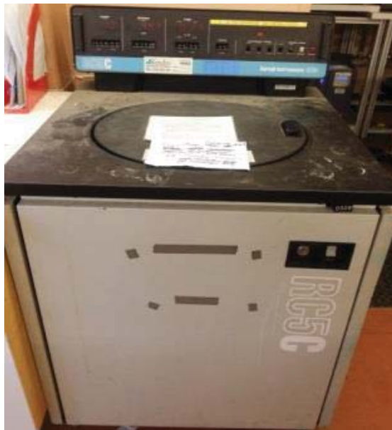
Figure 3.22: A Sorvall RC-5C from 1991 centrifuge
