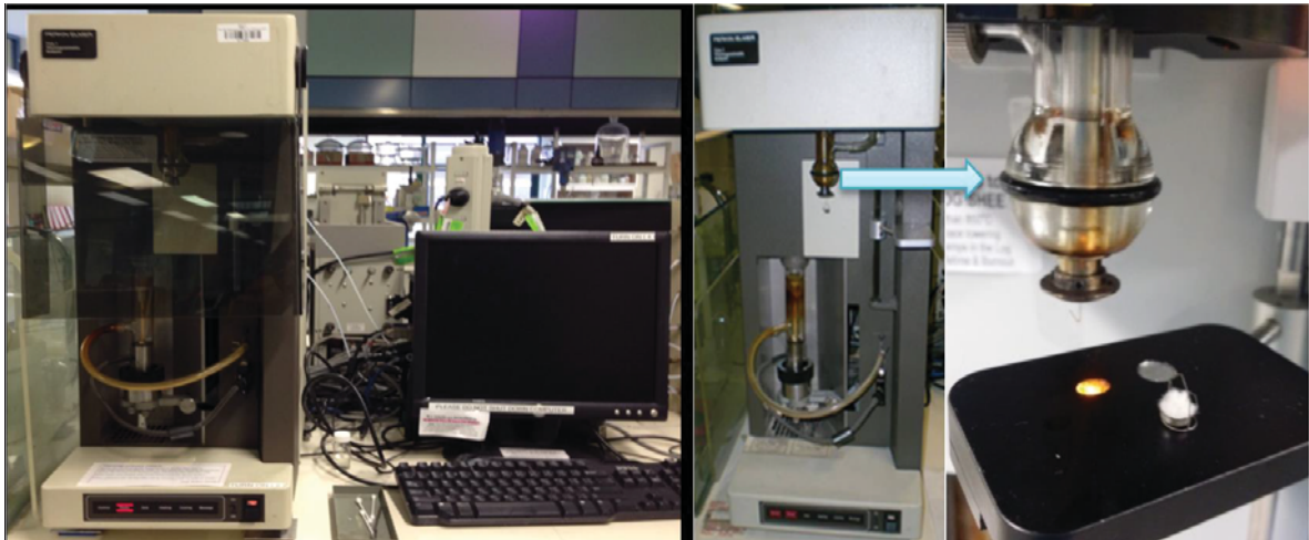
Figure 3.13: Perkin Elmer TGA 7 thermogravimetric analyser
