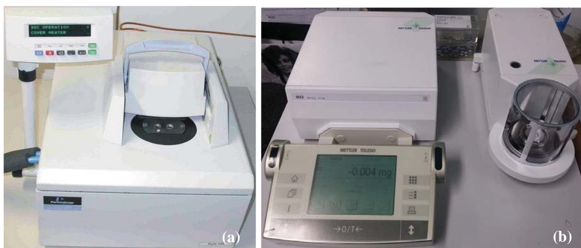
Figure 3.12: (a) PerkinElmer Pyris 1 differential scanning calorimeter (DSC) and (b) Mettler Toledo MX5
