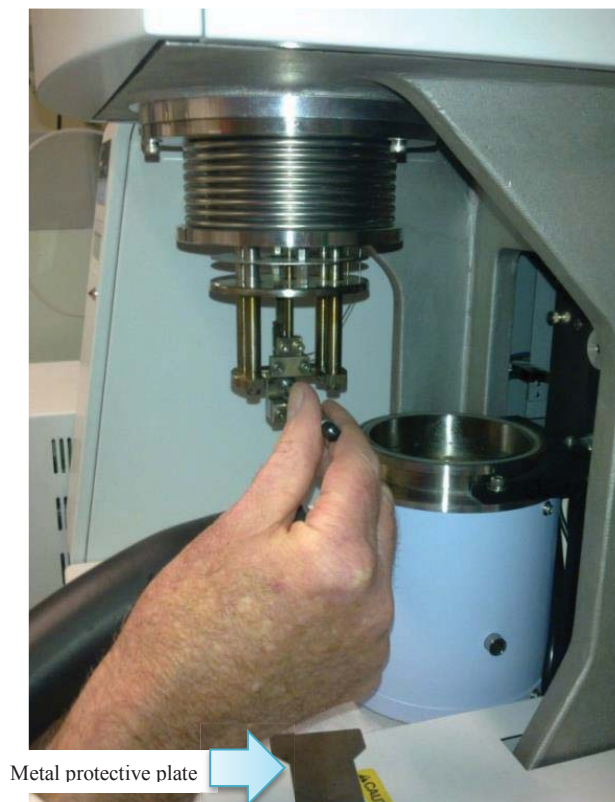
Figure 3.18: DMA showing mounting of a TPU/CFFs bio-composite (centre), heater unit (right-hand side) and metal protective plate (bottom) [18]
