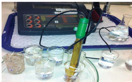
Figure 5.1: pH measurement of CFs rinsed water using pH HACH® SensION5™ Portable pH Meter
