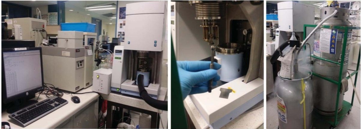
Figure 3.17: A PerkinElmer Pyris Diamond DMA 2003
