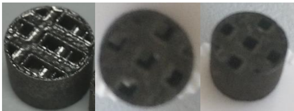
Figure 90 (Left) Unaltered 17-4 PH cylinder (Middle, Right) Ni on 17-4 PH cylinder after 550°C calcination & 700°C reduction Sample ID [E-c]
