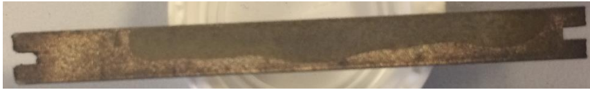
Figure 101 NiO/Al 2 O 3 on 17-4 PH plate after 550°C/4h calcination; Sample ID [A-p].
