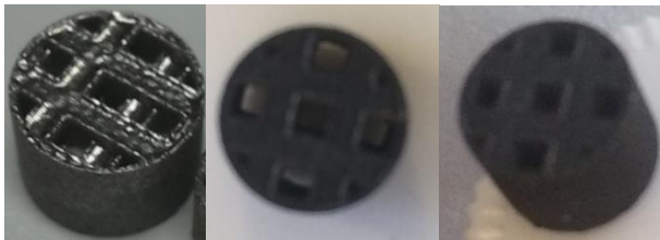
Figure 102 (Left) Unaltered 17-4 PH cylinder (Middle, Right) Ni/Al 2 O 3 on 17-4 PH cylinder after 550°C calcination, 700°C reduction & reaction; Sample ID [A-c]
