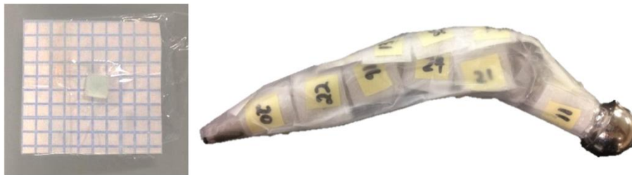
Figure 60: The left figure shows a 3 \times 3 mm TLD-100H chip. It is affixed to a small square of graph paper by plastic cling wrap which is held in place by double sided tape at the edges of the square. The right figure shows the graph paper squares with attached TLDs affixed to the hip prosthesis following irradiation.
