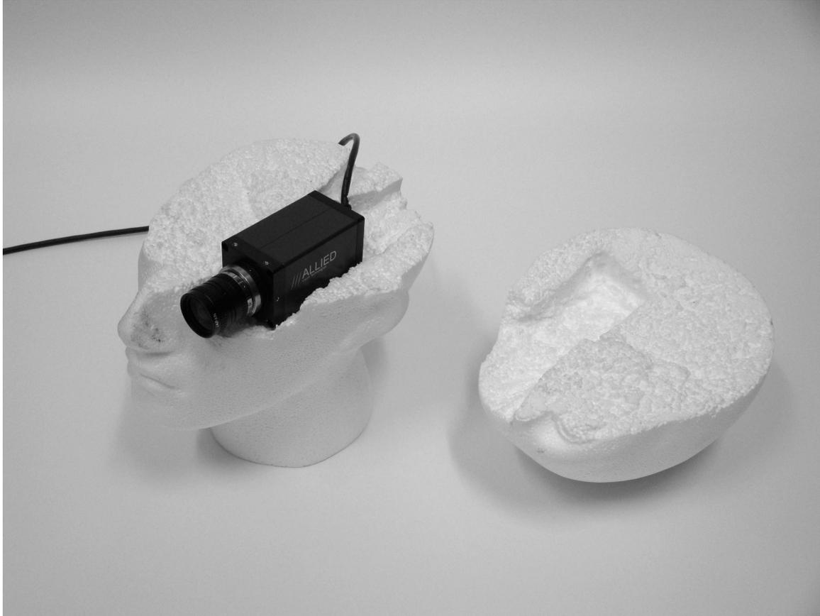
Figure 3: Mannequin head with camera in position.
