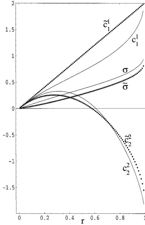
Figure 6. A comparison between the CRWs' self-induced phase speeds ( $c_1^1$  and  $c_2^2$ ) and the interaction coefficient  $\sigma$  obtained by the home-base method (solid lines as shown in Figs. 4(a) and (c)) and their approximate values (indicated by the dotted lines), as evaluated in section 2(c)(ii) using some simple CRW structure approximations:  $\tilde{c}_1^1 = 2r$ ;  $\tilde{c}_2^2 = z_2 - 2r^2$ ;  $\tilde{\sigma} = \{r e^{-z_2/(2r)}\}^{1/2}$ .
