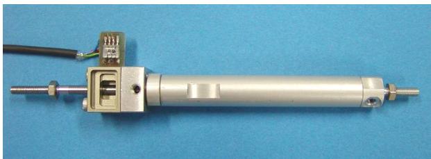
Figure 3. Intelligent cylinder and built-in sensor
