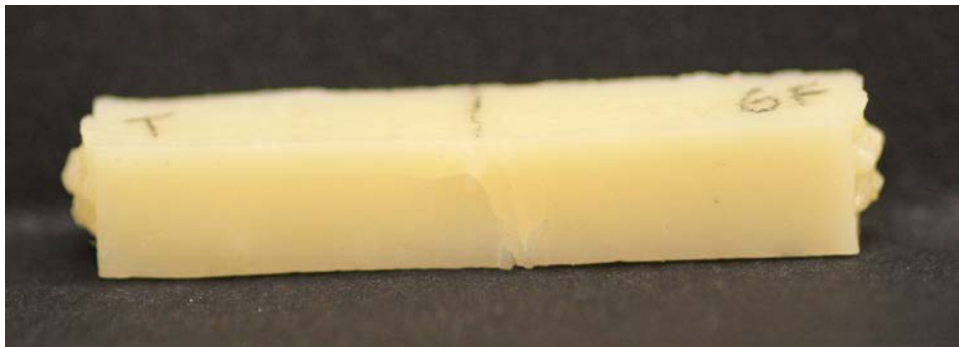
Figure 13: BAC resin with fractures and chipping on the tension side
