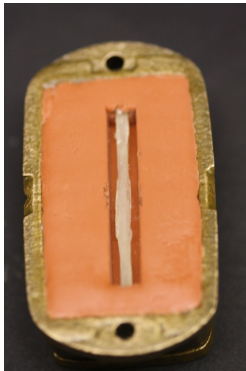
Figure 8: Impregnated glass fiber positioned within lateral slots
