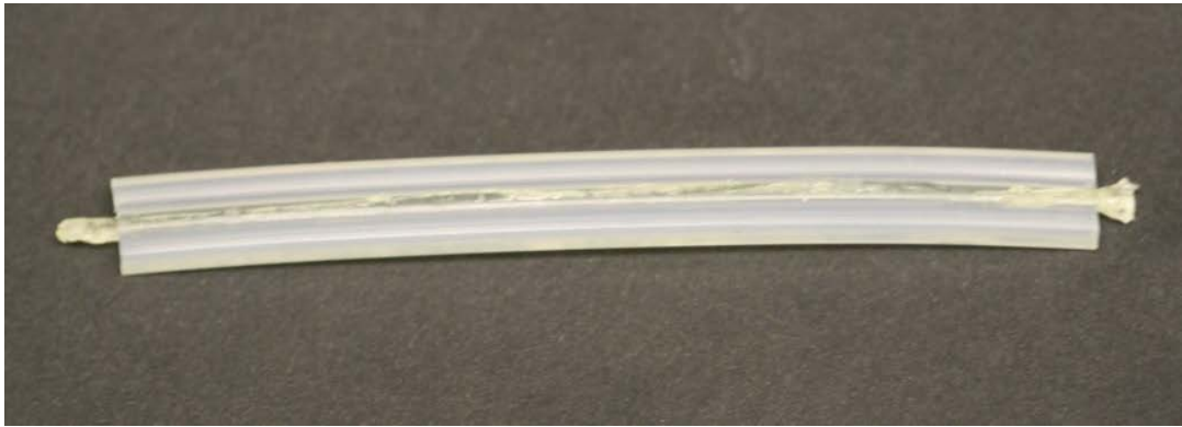
Figure 7: Impregnated glass fiber with clear silicone matrix
