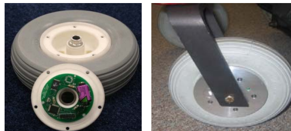
Figure 5.2. Power Wheelchair Data Logging Device
