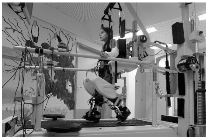
Figure 1 Robotic-assisted locomotion training of a 12-year-old girl with cerebral palsy on the driven gait orthosis (Lokomat®).
