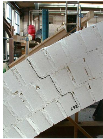
Figure 5. Hinges forming in the arch barrel at \frac{1}{4} span (left) and \frac{3}{4} span (right).
