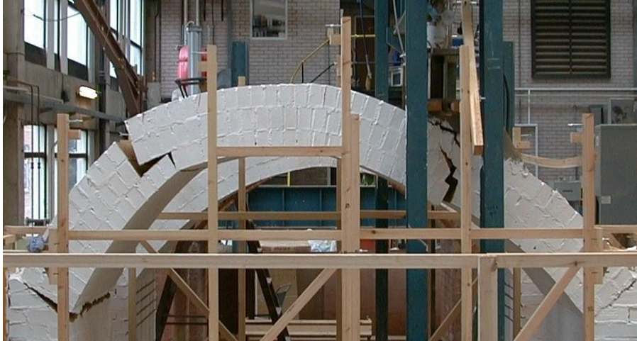
Figure 3. Arch 1 (unreinforced control) showing the 4-hinge collapse mechanism.
