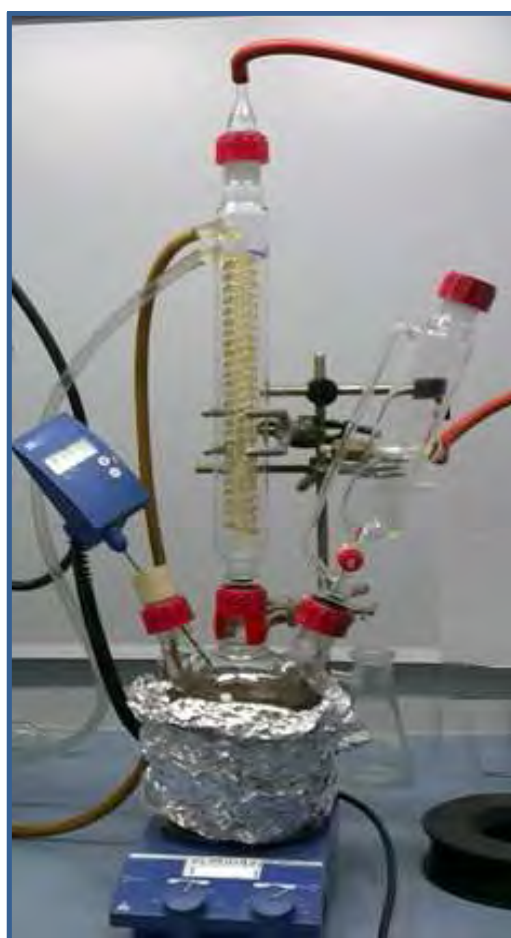
Figure II- 3: Synthesis of the ionic liquid was carried out in a round-bottom flask connected to a reflux condenser under constant nitrogen atmosphere.
