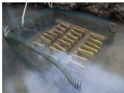
Figure 1: Artificial substrates (polyethylene plates) used for in situ production and collection of natural phototrophic biofilms (site M on the photography).
