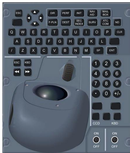
Figure 91. Exemple de Keyboard and Cursor Control Unit (KCCU)
