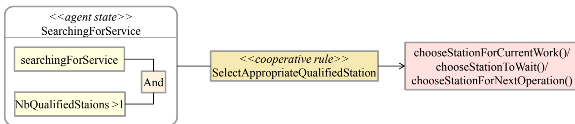
Figure 5.4 — The select appropriate qualified station Cooperative Rule for solving the stations concurrence NCS
