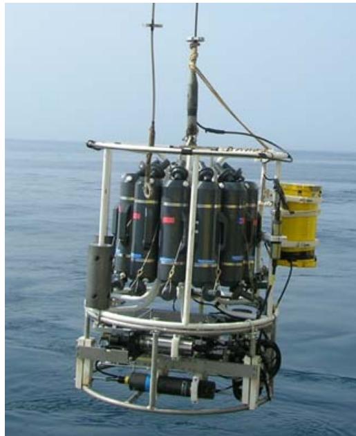
Figure 2.2: A picture of the CTD and rosette with Niskin bottles used onboard MOUTON 2007 survey. Grey containers are the Niskin bottles, yellow probe on the right is the LADCP, below are found all biogeochemical sensors.
