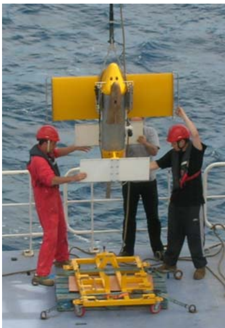
Figure 2.1: A picture of the Seasoar used onboard MOUTON 2007 survey. Towed behind the ship at 8 knots, it measures conductivity (salinity), temperature and pressure along a sinusoidal route in the water column.
