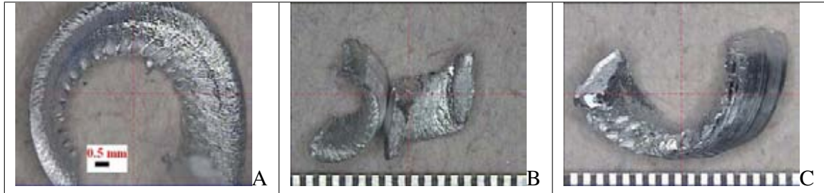
FIGURE 4.26 – Forme des copeaux, A. Plaquette O1, B. Plaquette S2, C. Plaquette S3.
