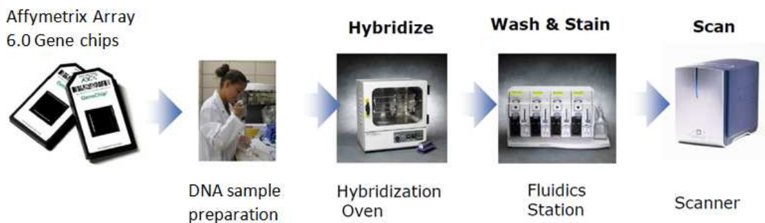
Fig.18. Affymetrix® Array 6.0 Gene Chip Work Flow with adapted equipment.
